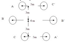
(ii)Determine the inductance per km of a double circuit 3 phase line as shown in Fig. The transmission line is transposed within each circuit and each circuit remains on its own side. The diameter of each conductor is 15mm. (May 2016)
